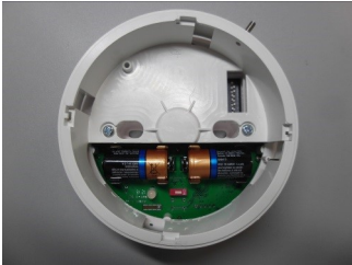
Picture 6 - primary and secondary batteries inserted
