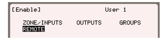
After selecting the remote option (and entering password as required) the user is presented with two options. To allow remote assistance select the option to "Allow remote access" as shown below.
