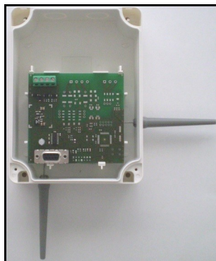
Figure 2 - Expander module inside view.
