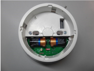
Picture 6 - primary and secondary batteries inserted
