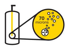
First, the Multi-Rotors located within the **system turn water into droplets of 70 micron** size by mixing it with air in a pre-set proportion.
