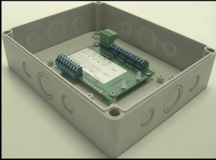
Picture 2 - multi-module's overview (without front cover)
