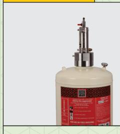
In cases where suppression systems protect smaller areas, a self-contained pulse mist-based system is used. Water is stored in nitrogen pressurised cylinders connected with detectors, pipes and nozzles. In an event of fire, the pressurised water is pushed through the specialised rotor and a little propellant (nitrogen) is also released into the water pipe via an air tube to create a bubbled mixture of water and nitrogen which arrives at the nozzle.
