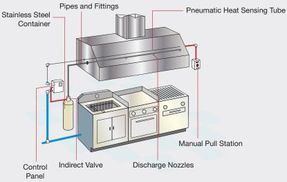
**Nozzles:** Specially designed nozzles that use minimum water and give maximum extinguishing power
