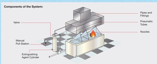
**Nozzles:** Specially designed nozzles that use minimum water and give maximum extinguishing power
