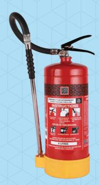
In commercial kitchens, the liberal use of fire and the presence of combustible substances make it easy for a fire to flare up. Designed to fight kitchen oil and fat fires, Ceasefire's Wet Chemical-based Fire Extinguisher uses an environmentally friendly foaming agent that blankets the flames, cuts down the supply of oxygen and cools the oil to below self-ignition point. Its de-greasing properties also ensure that the kitchen can be cleaned easily post a fire.
