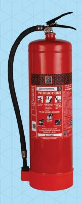
Ceasefire's watermist-based portable extinguisher is powered by Watermist. Once the system is triggered, a specially designed rotor within the mist generator mixes air and water in a pre-set proportion to generate Watermist. The mist is then propelled at the fire through a specially designed nozzle with a throw of 10 feet. The mist then quickly blankets the flames and brings down the temperature to below combustion levels.
